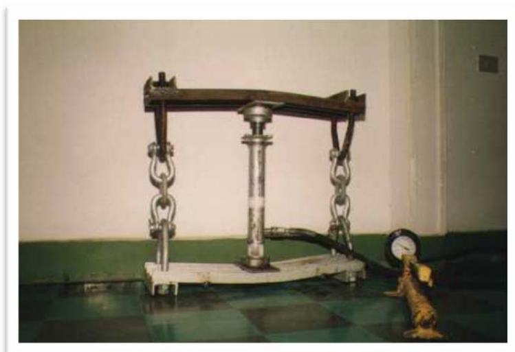
PLATE BEARING EQUIP.
