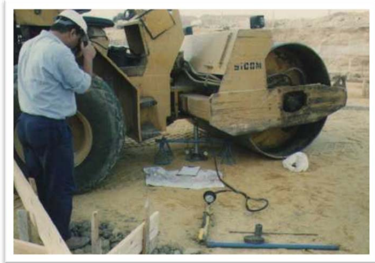
PLATE BEARING EQUIP.
